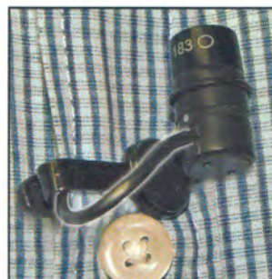
Figure 3 Loop cable back through tie bar to reduce cable noise.
